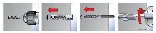
Instructions for placing anchors and bolts. Source: Fischer
