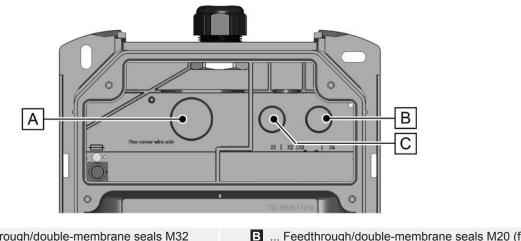
Feedthrough/double-membrane seals M32 (power supply line) **B** ... Feedthrough/double-membrane seals M20 (for control line/Ethernet)
