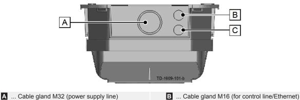
**C** ... Cable gland M16 (for control line/Ethernet)
