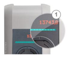
The optional dot matrix display (1) can display various information depending on the operating state (e.g. software version, energy meter status).
