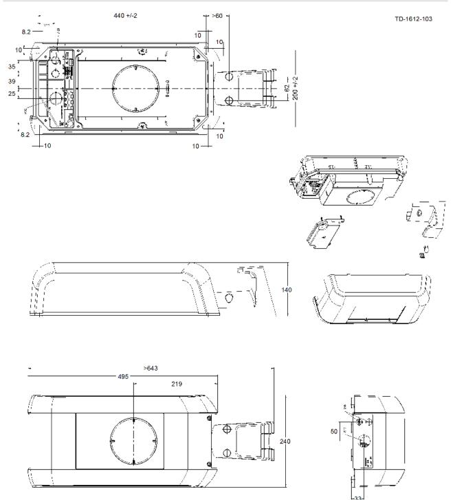
Figure 5-2: Dimensions in millimeters
